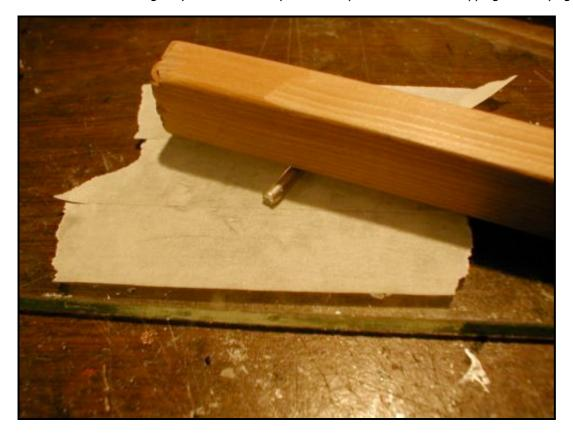
With the pieces straight, glue two pieces together with epoxy or super glue making sure they're flush at one end. My preference is super glue. But only glue one end. We do not want the entire length glued together. You will see why later.
