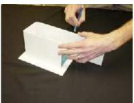
Here you can see how we are sizing the mold box right around the base of the clay. We simply score the plastic and bend it around the base. We then seal the inside of the mold box by smearing the clay tightly against the box. This ensures us the mold box will not leak. It is a good practice to double check this before pouring your rubber. An extra minute double checking the mold before pouring could save a costly mistake and a real mess.
