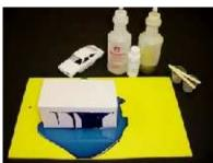
The Alumilite Regular has 90 second work time and a 3-7 minute demold time. With a thin walled car you will want to wait closer to the 7 minutes before demolding. The Alumilite Regular features a color change to at the 90 second point to notify you when the work time has ended. You can see the color difference in the blue as it begins to harden.
