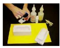
Now we are ready to pour our cast replica. We chose to add some blue dye to the resin to help it show up a little bit better. We simply mix equal amounts of the A side and B side of Alumilite Regular with a few drops of Alumilite's Blue dye. We mixed 2 oz of A and 2 oz of B. Even though the part only requires 2 oz total we use a little more to make sure it squishes properly and pushes all of the air bubbles up and out the seam line.
