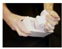
Here you can see the two halves of the mold seperating. We wanted to show you this shot, so you can see the advantages of having a flexible silicone (HS II) with an extremely high tear strength. You will not rip this mold when you demold it. Unfortunately, it is difficult to see the white car body inside the mold. The colors of the rubber and the car are just too close. But the car body remains inside the mold until you flex the bottom half of the mold and remove the original.
