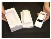
Here you can see the unharmed original car body and the perfect silicone mold that picked up every single detail of the original. You can also see in the front of the mold the locator that we put into the clay before we poured the rubber. Then when we poured the two silicone halves it provides us a mechanical locator to match or seat the mold properly when putting it back together.
