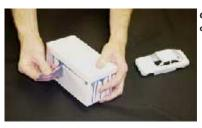
Once the material has hardened, simply peel off the excess material that was squished out of the mold.
