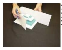
Once you have clayed up your original you need to make a mold box to contain the liquid silicone you are about to pour. We chose to use some corrugated plastic that is simply scored and bent around your base of clay. Your mold box should be approximately 1/4 to 3/8 of an inch away from your piece. You can use any nonporous material to make your mold box such as metal, Formica, plastic, wood, pvc, glossy side of posterboard, old yogurt or Cool Whip containers, etc.
