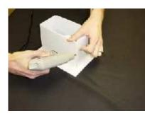
Here you can see we are using hot melt adhesive to glue and seal the seam of our mold box. We will also use the hot melt to seal all the edges of box to the base just in case the silicone were to seap down inbetween the box and the clay. The would prevent the silicone from leaking. You can also use super glue, caulk, epoxy, clay, tape, or any other material to seal your mold box shut. Just make sure it is sealed tightly.
