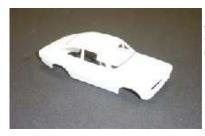
First we will start with an original that requires a two piece mold that will require male and female mold halves. This car works perfectly to demonstrate this because the exterior side will act as our female half of the mold (think of it upside down) and the male (squish) half of the mold will nestle down into the female side to give us the proper part thickness.
