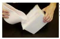
Once you have thoroughly coated the first half of the mold with mold release, you are ready to pour the second half. Mix the HS II silicone rubber and pour it into the mold box creating the second half of your mold. You can see in this picture we tilted the mold when we began to pour to make sure the silicone got underneath the deep front bumper.
