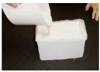
Once we knew we had the silicone underneath the bumper we simply put it back flat and finished pouring it. You can see the hot melt glue from the first half of the mold still on the edge of the mold box.
