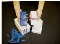
Here is a good picture of the original car along side of our perfectly cast replica. Now all we have to do is to trim out the window, wheel wells, and bumpers.
