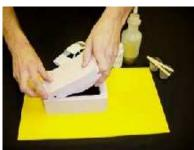
Then starting from the side with the locator, flex the silicone rubber and squish the top half of the mold into the bottom half. Important note: When we use the term squish, we do not mean to apply force. We simply mean to set the male side of the mold into the female cavity to allow the excess resin to be squished out the seam line.
