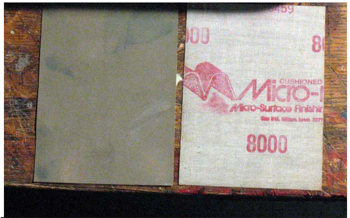
Here is one brand of 8000 and 12000 grit sanding material. It is washable and works well with electrical parts
