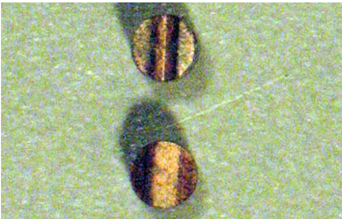
Motor brushes. The top one is the bottom view, the lower one, the top of the brush. Note the groove in the top brush. This helps prevent the brush from rotating.
